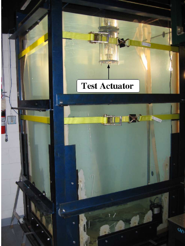
Fig. 5. Thruster-testing tank developed for this experiment. The tank is approximately 1 \text{ m} \times 1.3 \text{ m} \times 2.3 \text{ m} .
